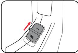
2. Push the switch downwards for a Continuous Shot adjustment. Pull and hold the trigger with its safety striker tip against the workpiece. It will now shoot every time the tip is depressed until the trigger is released.
