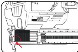
**WARNING!** THIS JAM RELEASE LATCH SHOULD 'CLICK' SHUT SECURELY BEFORE USE TO PREVENT ACCIDENTAL MISFIRING.
