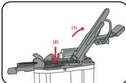
3. Check for any jammed nails in the magazine.
