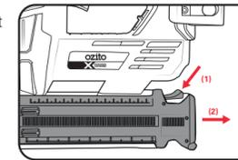
**Note:** Make sure the jam release latch is closed at all times except when troubleshooting.
