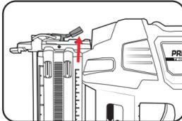
2. Open the jam release latch. (1) Using a pair of pliers, carefully remove any jammed nails. (2)
