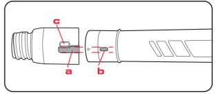
2. Rotate the adaptor to lock the raised tab (b) in opening (c).
