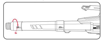
WARNING: THE ADAPTOR MUST BE TURNED AS FAR AS IT WILL GO AND LOCK INTO PLACE TO ENSURE IT IS FIRMLY SECURED IN POSITION. 3. Screw the 400mm Extension onto the Adaptor.
