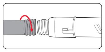
4. Depending on your requirements, screw on more 400mm extensions or the Gutter Nozzle.
