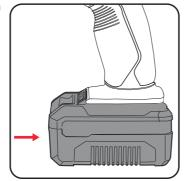
2. To remove, (a) press and hold the battery release button (b) release tab and then slide out.
