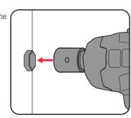
5. Slowly increase pressure on trigger to appropriate torque for circumstances until bolt is tightened.
