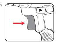
2. Release the variable speed trigger to stop the wrench.
