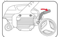
3. To increase the cutting depth pull the lever out and move it up a notch, towards the front of the unit.
