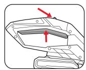
3. Slowly raise the handle to lower the cutting blade within the edge to be cut.
