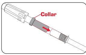
2. Slide the shaft lock over the collar onto the threaded section and screw tight.
