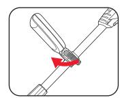
2. Adjust the handle into the most comfortable position, then lock in place with the lever.
