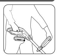
2. To start the edger, press and hold the lock-off switch forward.
