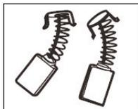
When the carbon brushes wear out, the sander will spark and/or stop. Discontinue use as soon as this happens. They should be replaced prior to recommencing use of the sander. Carbon brushes are a wearing component of the sander therefore not covered under warranty. Continuing to use the sander when carbon brushes need to be replaced may cause permanent damage to the sander. Carbon brushes
