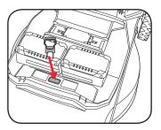
WARNING! ALWAYS ENSURE THE SAFETY KEY AND ALL BATTERIES ARE REMOVED WHEN NOT IN USE.
