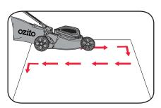
When mowing long grass be sure to not overload the motor. First cut with the highest cutting height and then to the desired height. This will help reduce the load.
