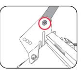
2. There are three holes remaining in each bracket, select the appropriate hole for the height of the user.
