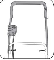
2. Secure knobs over the protruding ends of the bolts.
