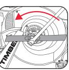
2. Remove the blade bolt and blade.
