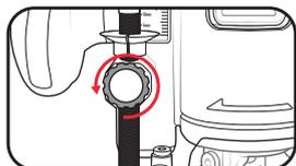
7. Then press and hold the lock button. The depth adjuster should drop and touch the end stop. This is the 0 position for the router bit where no material is removed when the plunge router is lowered.
