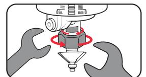
**WARNING!** THE SPINDLE LOCK IS NOT ALLOWED TO BE USED FOR TIGHTENING WITH THE SPANNER. TIGHTEN THE CLAMP NUT USING THE TWO SPANNERS.
