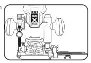
1. Loosen the guide mount screw.
