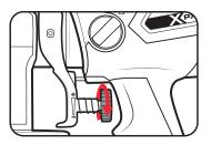
2. To increase the amount sprayed in one go, turn the Dial anticlockwise.
