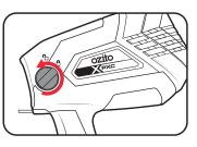
Note: Ensure the Spray Head and Spray Gun body are aligned correctly for proper fitting.
