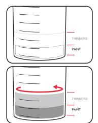
Pour the required paint and thinners through a filter into a mixing cup and mix thoroughly.
