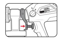
2. Release the On/Off Trigger to stop spraying.
