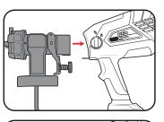
3. Press the Spray Head Locking Knob and turn it clockwise to the locked position to secure the Spray Head in position.
