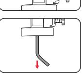
4. Dip a clean rag in water/solvent and clean the nozzle lid, Nozzle parts, Spray Gun housing, rear of the Paint Head and Suction Tube.
