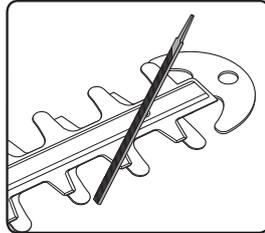
**Note:** Do not operate your hedge trimmer with dull or damaged cutting blades. This may cause overload and will give unsatisfactory cutting results.
