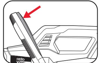
2. To start the hedge trimmer, squeeze the on/off trigger.
