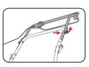
2. Secure in place with washer and quick-release lever.
