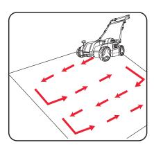
For optimum operation, always scarify in a straight line; do not swing the scarifier from side to side.
