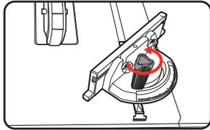
3. Rotate the mitre gauge to the desired angle using the mitre scale.
