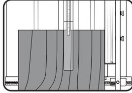
When cutting thin materials, loosen the 2 thumbscrews on the rip fence and slide the stop rail onto the bolts before tightening everything into place.
