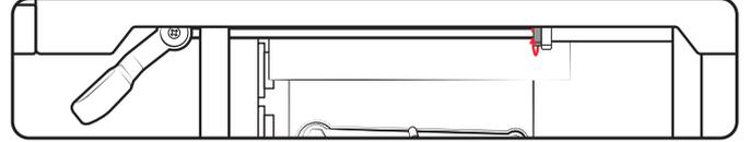
2. Adjust the threaded sleeve by turning it in or out until the desired clamping force is reached.
