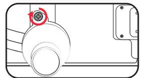
3. Replace the screw to lock the adaptor in place.
