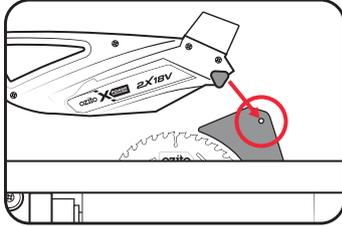
**Note:** the blade guard must be able to move freely, adjust if necessary.
