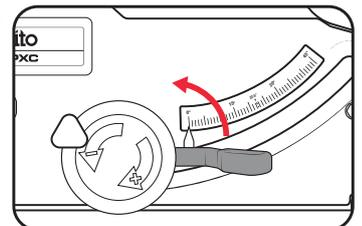
2. Slide the adjustment wheel to the desired angle using the bevel scale as a guide.
