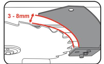
5. Re-tighten the riving knife bolt.
