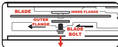
**Note:** Ensure that the inner flange is attached to the motor shaft.
