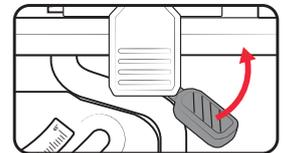
2. Extend the table so that the workpiece is properly supported.
