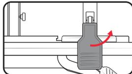
2. Slide the rip fence to the desired dimension using the scale on the guide rail.
