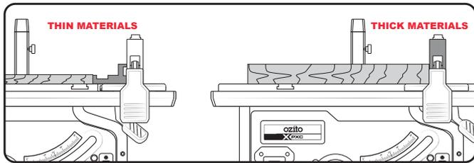
When cutting thicker materials, remove the stop rail and bolt assemblies from the rip fence (if attached).
