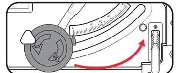
3. Secure the bevel angle by flipping the bevel lock down and right.
