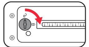
6. Replace the table insert and use the spanner to lock it in place.
