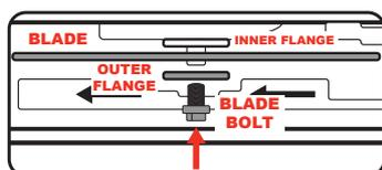
7. Refit and set the riving knife, table insert and blade guard. Ensure the blade direction matches the arrow direction indicated on the riving knife & blade guard.
