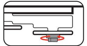
4. Insert the riving knife behind the plate, leaving a 3-8mm gap between the riving knife and blade teeth.
