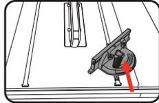
2. Loosen the screw to adjust the mitre angle.
