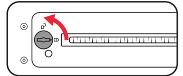
2. Raise the blade to its highest position by turning the adjustment wheel clockwise.
