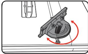
4. Lock the mitre angle by tightening the screw.
