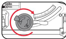
2. Remove the blade guard by undoing the screw.
