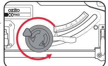
2. To raise the blade for a larger depth of cut, rotate the adjustment wheel clockwise.
