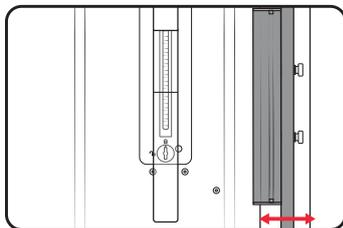
3. Press the rip fence lever down to lock it in position.
