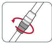
2. Extend to the desired height and then retighten the shaft adjustment collar to secure in place.
