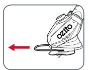
2. Align the tabs of the safety guard with the recess in the back of the cutter head.
