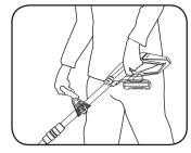
3 To turn on squeeze the on/off trigger whilst holding the lock-off button down. 4. Move the grass trimmer into the grass to allow it to cut.
