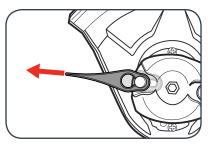
3. To remove the blade push the blade towards the centre of the spindle and then slide off.
