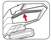
To stop the trimmer, release the On/Off trigger.
