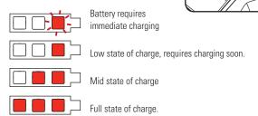
**Note:** The battery needs to be removed from the tool to check the state of charge.
