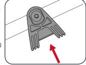
2. Place the adjustable handle on the mounting bracket, then pass the screw with washer through the mounting bracket and onto the adjustable handle lever.
