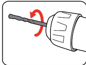
5. Check SDS+ accessory is locked. Try to pull it out. Note: It should have approximately 10 – 20mm movement. This is normal.
