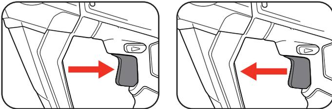
**Note:** The more the variable speed trigger is depressed, the faster the drill bit will rotate.
