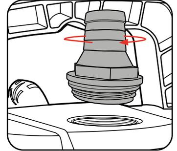
2. Securely attach the hose/tube/pipe to the Hose Adaptor, fit hose clamps (not included) if you are using flexible hose or tube, and tighten well.
