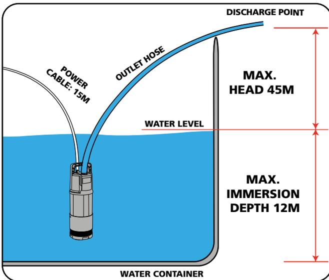
3. Ensure the pump is placed on a flat and level surface, there are no obstructions to the suction base and it is clear of mud or sediment.
