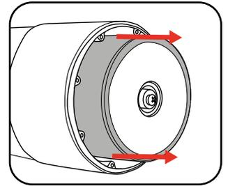
5. Clean all parts removed and the exposed base of the pump with clean water.
