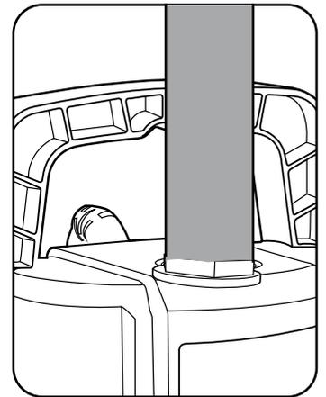
**NOTE:** The maximum pumping rate is possible only with the largest possible line diameter; if smaller hoses or pipes are connected, the pumping rate will be reduced.
