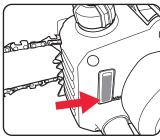
MARNING: NEVER START WORK UNLESS THE CHAIN AND BAR ARE LUBRICATED.
