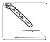
**Note:** Chain bar oil may leak if the chainsaw is left for long periods. This is normal. If the machine is to be left unused for an extended time, drain the oil from the chainsaw. Refill before use.
