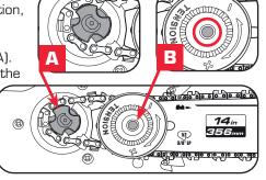
Attach the side cover and secure it with the side cover lock. Do not fully tighten the guide bar lock knob until after adjusting the chain tension.
