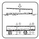
holding it off the ground, first saw down from the top one-third through the log then finish by sawing up from the bottom.
