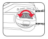
For the correct chain tension, firmly pull up on the chain at the middle of the top of the exposed guide bar. When the chain is pulled up to its highest point, the bottom tip of the links should only just stay in the track [middle of the guide bar].
