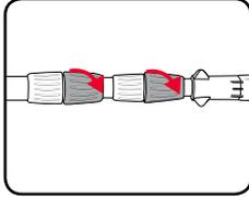
2. Pull out the telescopic tubes to suit the required working height.
