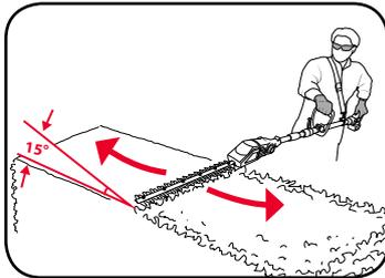
**Note:** Do not use the pole hedge trimmer for cutting stems greater than 12mm. Use the trimmer only for cutting normal shrubbery found around houses and buildings.
