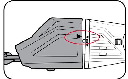
2. (a) Press the trimmer head against the motor head. This will cause the lock button to be pushed to the right.
