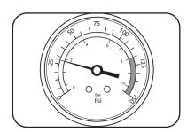
3 Once the compressor is switched on and the item is being inflated, the pressure reading will increase on the pressure gauge.
