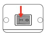
4 Once the pressure gauge reads the required pressure, switch the compressor off.
