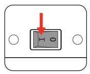
2 Press the on/off switch into the off position "0" to stop the compressor.
