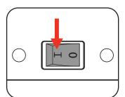
5 Switch the compressor off and remove the adaptor from the inflated item.
