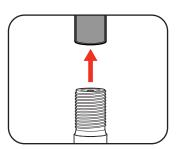
2 Attach the air hose by screwing the end of the hose in a clockwise direction.
