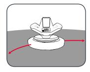
**Note:** Do not apply excessive force to the polisher. Allow the polisher to do the work.
