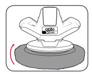
2 Insert the battery, hold the polisher on the surface and start the tool.
