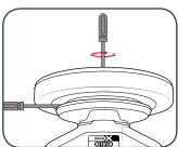
3 Reinstall the foam pad by rotating the securing screw clockwise.
