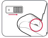
3 Allow the motor to reach maximum speed and move the polisher using long sweeping strokes in a crisscross pattern.
