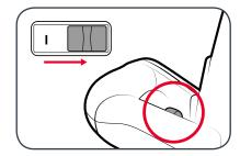
2 To stop operation, press the on/off switch into the off position "0".
