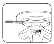
2 Using a phillips screwdriver remove the screw holding the foam pad, by turning it anticlockwise.
