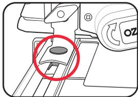
2. Slide the guide to the required position and tighten the wingnut.
