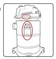
2. Hook the securing clips over the lip of the motor unit and then press lower end of the clips against the sides of the tank to lock them in place.
