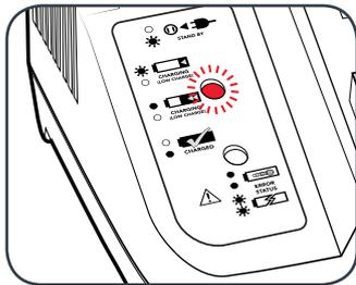
5. The green LED will illuminate once the battery is fully charged.
