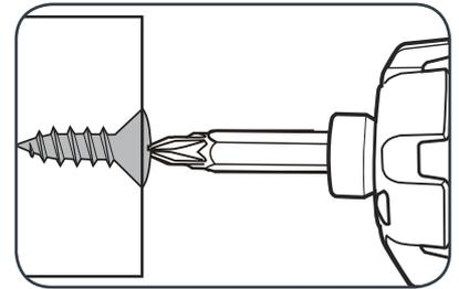
**Note:** Do not force the driver or apply side pressure to elongate the hole. Let the impact driver do the work.
