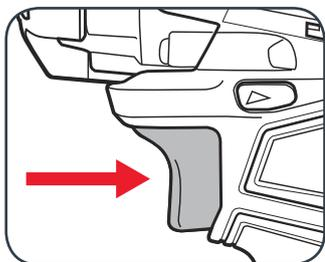
2 Release the variable speed trigger to stop the driver.
