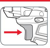
2 Check the forward/reverse lever is on desired setting.
