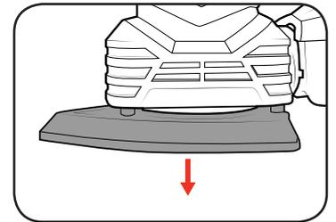
**Note:** The base aligning pins can sometimes get stuck in the base of the tool.
