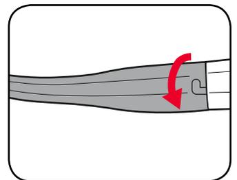
5. To remove blower tube extension, rotate in anti-clockwise direction.
