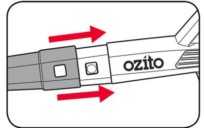
3. Align the blower tube extension with the end of the split blower tube and slide into place.
