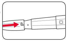
4. To lock into place, rotate extension in clockwise direction until extension clicks into place.
