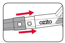
3. Align the blower tube extension with the end of the split blower tube and slide into place.
