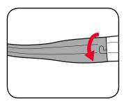
5. To remove blower tube extension, rotate in anti-clockwise direction.
