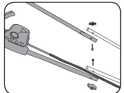
3. Secure in place by screwing the handle securing knobs over the protruding ends of the bolts.
