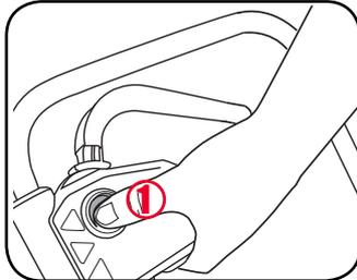
2. Pull the start/stop lever towards the handle to start the mower and then release the lock-off button.
