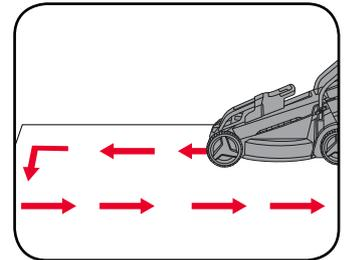
For optimum grass collection, always mow in a straight line; do not swing the lawn mower from side to side.
