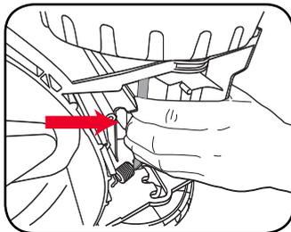
**Note:** Make sure that front, back, left & right wheels are located in the same cutting height adjustment position.
