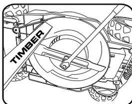
**NOTE:** A piece of timber will assist in holding the blade while removing or tightening the blade bolt.
