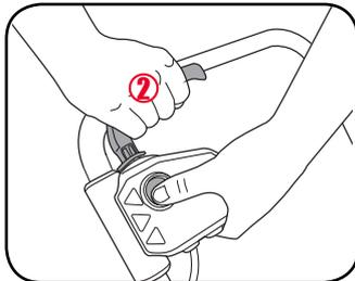
3. Release the start/stop lever to stop the mower.
