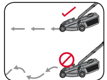
When mowing long grass be sure to not overload the motor. First cut with the highest cutting height and then to the desired height. This will help reduce the load.
