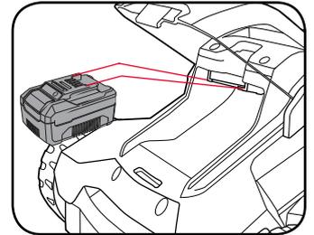
3. Insert the safety key. (If the mower is not going to be used immediately, do not insert the safety key.)
