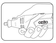
5 Gently apply the tip of the accessory to the work piece.
