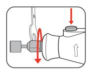
Note: Always ensure the shaft of the accessory bit is fully inserted into the collet and is tightened correctly before use.
