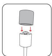
3 Tighten the screw until the sanding drum sleeve is secured.
