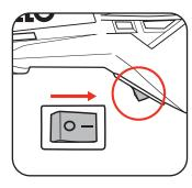
2 To turn off, push the on/off switch to the off position "0".
