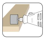
WARNING PLACING EXCESSIVE LOAD ON THE ROTARY TOOL WHILE IT IS RUNNING AT LOW SPEEDS MAY CAUSE IT TO OVERHEAT AND THE MOTOR TO FAIL.
