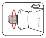
5 Fully insert the shaft of the accessory into the collet.
