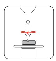
**Note:** Do not over-tighten the screw as it could result in damage to the cutting disc.
