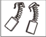
When the carbon brushes wear out, the angle grinder will spark and/or stop. Discontinue use as soon as this happens. They should be replaced prior to recommencing use of the angle grinder. Carbon brushes are a wearing component of the angle grinder therefore not covered under warranty. Continuing to use the angle grinder when carbon brushes need to be replaced may cause permanent
