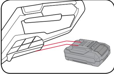
2. To remove, press and hold the battery release tab and then slide out.
