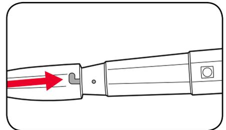
4. To lock into place, rotate extension in clockwise direction until extension clicks into place.
