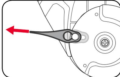
3. To remove the blade push the blade towards the centre of the spindle and then slide off.
