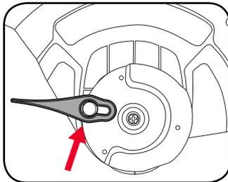
2. Pull the blade outwards so that the small hole is fitted into the mount.
