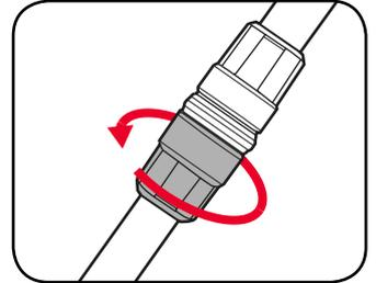
2. Extend to the desired height and then retighten the shaft adjustment collar to secure in place.
