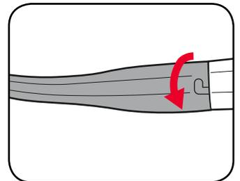
5. To remove blower tube extension, rotate in anti-clockwise direction.
