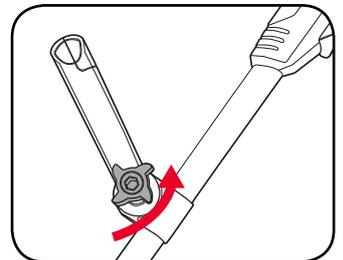
2. Rotate the handle into the desired position and then tighten the locking knob.
