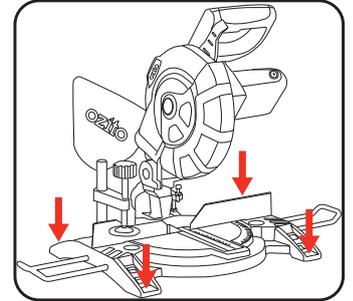
**Note:** If required, the Mitre Saw can be mounted onto a 13mm piece (or thicker) of plywood which can then be clamped to the work bench or mitre saw stand. This provides the flexibility to transport the Mitre Saw to other work areas.
