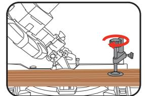
**WARNING!** ENSURE THE MATERIAL IS SECURELY CLAMPED BEFORE MAKING ANY CUTS. FAILURE TO SECURE THE MATERIAL MAY CAUSE THE WORKPIECE TO FLY OFF AND CAUSE PERSONAL INJURY.
