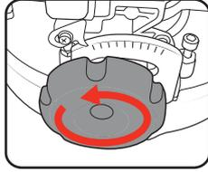
2. Tilt the cutting head to the desired bevel angle.
