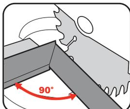
**Note:** The square must contact the blade, not the teeth, for an accurate reading.
