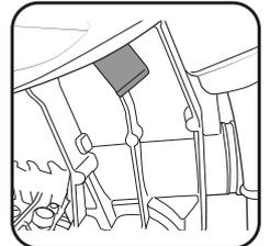
**Note:** The spindle lock button holds the blade in place when using the 6mm Hex Key to change the blade.
