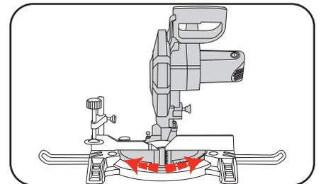
**Note:** The mitre table features positive click stops at 0°, 5°, 10°, 15°, 22.5°, 30°, 35°, 40° and 45° for quick setting of common mitre angles.
