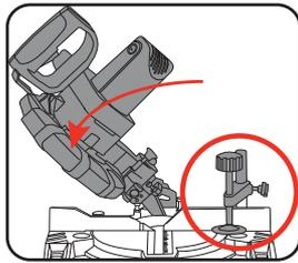
**Note:** The material clamp cannot be used on the left side of the mitre saw whilst bevel cutting.
