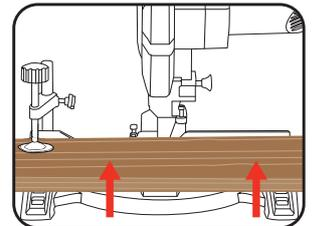
**Note:** If the workpiece is warped, ensure the concave (curves inward) side is against the rear fence.
