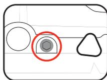
2. Flip the safety guard lever, lower the cutting head and hold it in place using the lock down pin.
