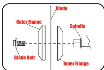
**Note:** Use a rubber mallet to tap the blade off if it is stuck on the tool.
