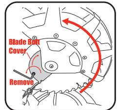
4. Swing the blade bolt cover up and out of the way to reveal the bolt head in the centre of the blade.
