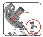
3. Tighten the bevel lock to lock the angle in place.
