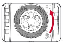
2 For a wide beam, rotate the beam setting dial clockwise " 글 p".
