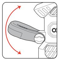
Turn handle locking knob clockwise to secure handle in desired position.
