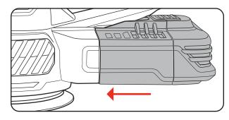
2. To remove, pull the dust canister away from the extraction port.
