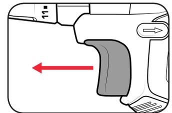
**Note:** The more the variable speed trigger is depressed, the faster the drill bit will rotate.
