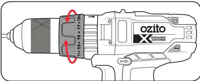
**Note:** Selecting a higher torque setting will allow the drill to use more torque to drive the screw in or out. To prevent damaging the screw head, it is recommended to start at a low torque setting and increase as necessary.
