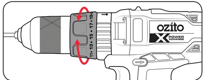
**Note:** Selecting a higher torque setting will allow the drill to use more torque to drive the screw in or out. To prevent damaging the screw head, it is recommended to start at a low torque setting and increase as necessary.
