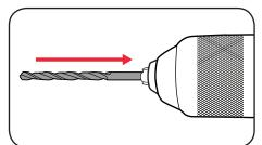
3 Tighten the chuck by turning it clockwise.
