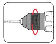
4 Pull on the bit to ensure it is firmly secured.
