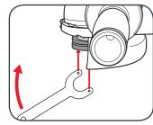
3 Remove the flange and replace the grinding disc on the spindle.
