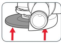
4 Screw the flange back onto the spindle and tighten using the pin wrench while holding the spindle lock down.
