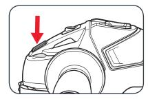
2 Using the pin wrench loosen the flange by rotating it anti-clockwise.
