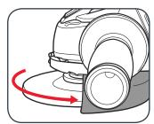
3 Tighten the safety guard locking screw to secure in position.
