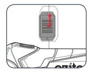
2 To turn off, slide the lock-on switch back and to the left.
