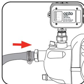
**Note:** The suction pipe should have an internal diameter of at least 25.4mm (1"); it must be kink resistant and suitable for pump use. Ensure the input hose or pipe is not restricted in any way.
