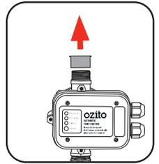
2. Wrap the discharge outlet with Teflon tape.
