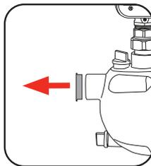
3. Insert 1" male threaded adaptor (not included). Tighten firmly with a spanner (not included).
