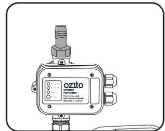
4. Securely attach the output hose or pipe (not included) to the other end of the adaptor. Ensure you have the correct diameter hose or pipe that is compatible with your water discharge application.
