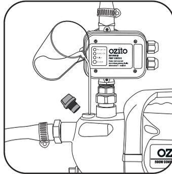
4. Fully open any (shut-off mechanisms, spray nozzles, valves, etc. in the pressure line) so that the air can escape without obstruction.
