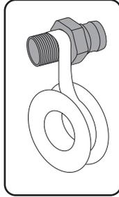
2. Remove the plastic protection cover from the suction inlet.
