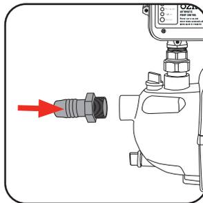
4. Securely attach the input hose or pipe (not included) to the other end of the adaptor. Ensure you have the correct diameter hose or pipe that is compatible with your water drawing source.
