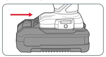
2 To remove, press and hold the battery release tab and pull the battery away from torch.
