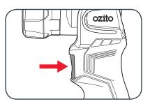
2 To turn the torch off, press the on/off switch again.
