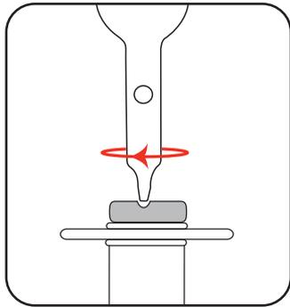
**Note:** Do not over-tighten the screw as it could result in damage to the cutting disc.
