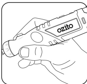
4 For heavy work like cutting or grinding, hold the rotary tool in the palm of your hand.
