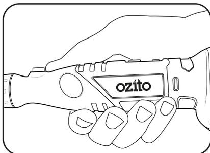
5 Gently apply the tip of the accessory to the work piece.
