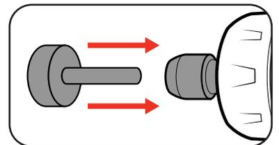
**Note:** The supplied collet will fit 3.2mm bits when fully open. When fully tightened it can reduce to hold 2.3mm bits.
