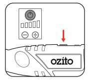
2 To turn off, push the on/off switch.
