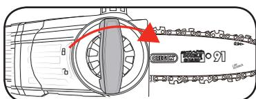
**Note:** Only tighten the chain cover locking knob securely once the chain tension has been adjusted (see: Tensioning the chain.)
