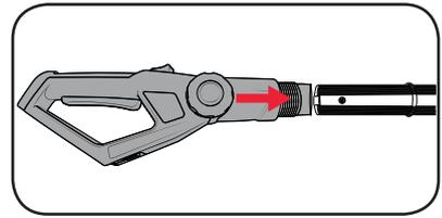
2. Screw tight with the assembly nut.
