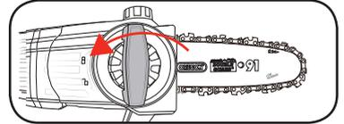
**CAUTION: IF YOU TRY TO ROTATE THE CHAIN TENSIONING ADJUSTMENT DIAL WHILST THE CHAIN COVER LOCK IS TIGHT, IT WILL RESULT IN THE CHAIN NOT LOOSENING AND POSSIBLE DAMAGE TO THE MECHANISM.**
