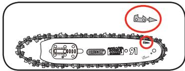
**IMPORTANT: IF THE CHAIN IS INSTALLED BACKWARDS (CHAIN CUTTERS ARE FACING IN THE OPPOSITE DIRECTION OF ROTATION) THE POLE PRUNER WILL VIBRATE EXCESSIVELY AND NOT CUT.**
