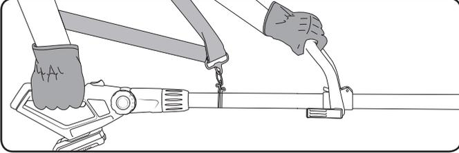
2. Slide the switch lock (a) to the front with your thumb and hold, then squeeze the trigger switch (b).
