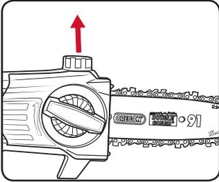
2. Fill the tank with chain bar oil. The capacity of the chain oil tank is 125ml. Do not over fill.
