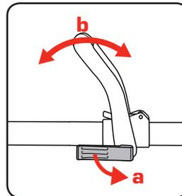
2. (a) Open the mounting bracket lever and (b) slide the auxiliary handle, close to lock into position.
