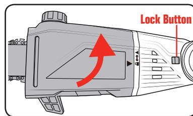
2. The pruner head will lock onto the motor head and is then secured in place.
