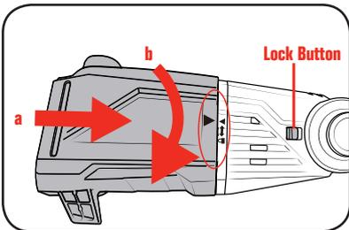
**Note:** The Lock Button will “CLICK” back to the left (original position) when the pruner head is correctly secured in place.
