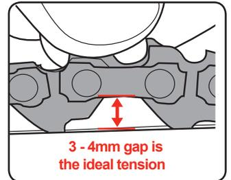
3. After the chain has been accurately tensioned, lock the guide bar in place with the chain cover locking knob.
