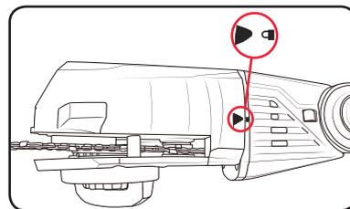
**Note:** The Lock Button will "CLICK" back to the left (original position) when the pruner head is correctly secured in place.
