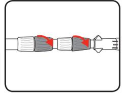
2. Pull out the telescopic tubes to suit the required working height.
