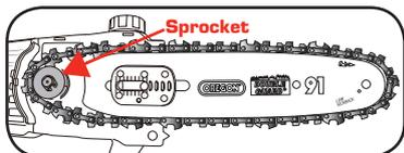
4. Re-mount and finger-tighten the side cover with the chain cover lock.
