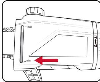
4. Always fill oil tank when the oil level is below the minimum mark on the oil level window.
