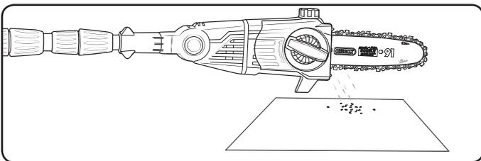
**Note:** Chain bar oil may leak if the tool is left for long periods. This is normal. If the tool is to be left unused for an extended time, drain the oil from the tool. Refill before use.
