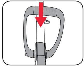
2. Pass the bolt through the auxiliary handle and screw the lever to the end of the bolt.
