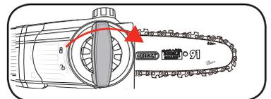
**Note:** Proper tension of the chain is extremely important and must be checked before starting, as well as during any cutting operation. Taking the time to make adjustments to the chain will result in improved cutting performance and prolonged chain life.
