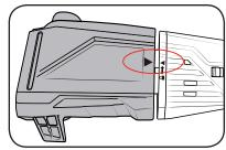
(a) Press the pruner head against the motor head. This will cause the lock button to be pushed to the right.
