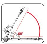
When removing branches, hold the pruner at an angle ranging from a maximum 60° to horizontal in order to avoid being struck by a falling branch.
