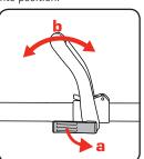
2. (a) Open the mounting bracket lever and (b) slide the auxiliary handle into the required position, close to lock into position.
