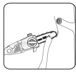
At the end of the cut, the weight of the pruner suddenly increases for the user, because it is no longer supported on the branch. There is the risk of losing control of the pruner.
