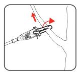
Only pull the pruner out of the cut with the chain running. By doing so, you can prevent it from getting jammed.
