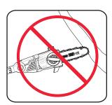
Do not saw with the tip of the guide bar. This could lead to kick back and possible injury.
