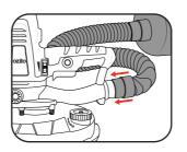
2 To remove the dust bag and hose, pull the end of the hose off the tools dust port.
