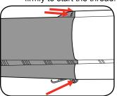
4 Secure in place with the 2 remaining 24mm screws and nuts.
