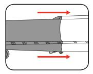
3 Feed the top of the assembled tubes into the blower housing first, then squeeze the bottom to fit.
