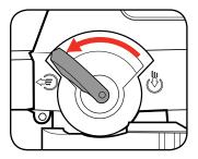
2 To select the vacuuming/ mulching function move the lever hard right to the vacuuming icon.
