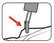
2 To unclip the blower, press either side of the buckle.
