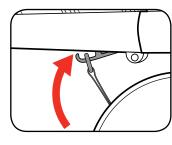
2 Attach the plastic connector at the top of the collection bag to the outlet in the housing.
