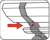
Secure the tubes with the 6 supplied 55mm long screw
