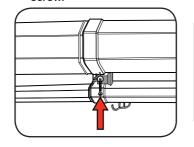
5 Slide the assembled tubes into the motor housing.
