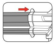
2 Insert the large lower tube into the matching upper tube and push together until they are connected firmly.
