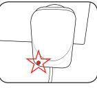
2 With the battery sitting on a flat surface, align the raised ribs on the battery with the recess in the charging cradle and slide onto the battery ensuring a firm connection.
