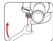
3 Remove the flange and replace the grinding disc on the spindle.
