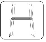
3 Once aligned, insert small bolts into the 2 aligned holes at both sides of the lower support. Insert the bolt from the outside and fit a small washer, spring washer and nut onto each bolt to secure (only hand tight at this initial stage).
