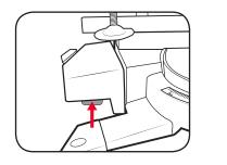
2 Slide the extensio support to the desired location and then release the locking lever to secure in position.
